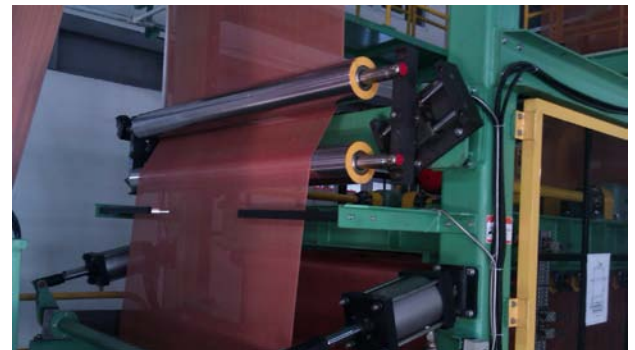
End Pivot Guider EPMP-TR(Double) is used on a Rubber Calender Machine
